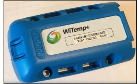
The WiTemp+ also supports the installation of a single 1-Wire temperatures sensor. This is accomplished by wiring the data wire to the port on the left and the common wire to middle port on the WiTemp+.
