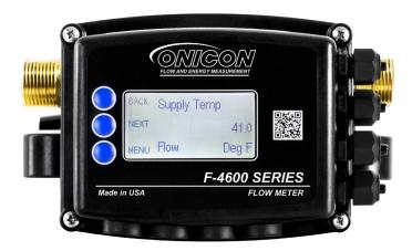
When provided with a display, the F-4600 features an IP65 enclosure. Field wiring connections are made to internal terminal blocks through the 4 cable glands provided.
