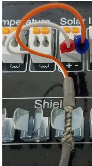
Figure 20: Solar irradiance sensor shield connection
