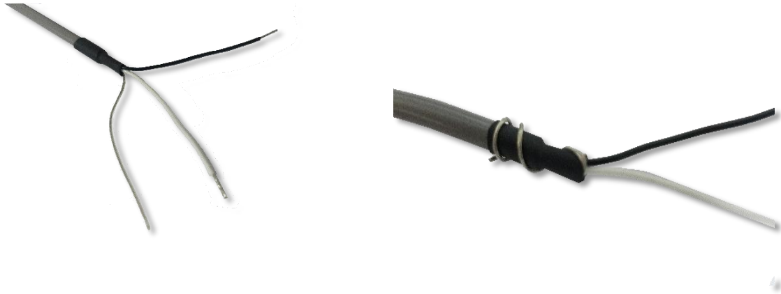
Figure 17: Typical BOM wire end and wire end with wrapped shield
